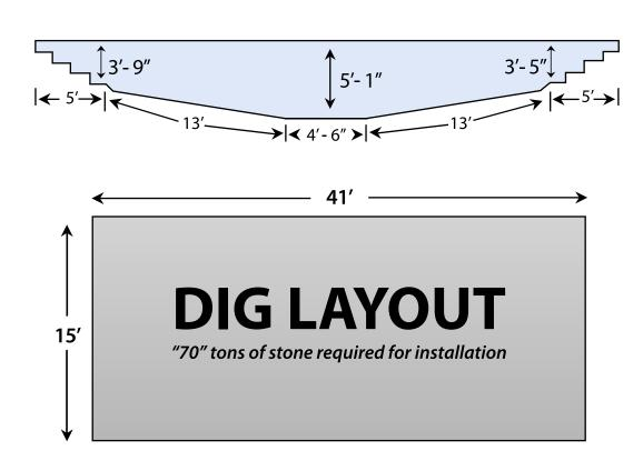
It is important to have your excavator call to review the Dig Diagram prior to excavation. All dimensions are approximate. A 3" over dig must be added to the botom for stone, along with a 2' by 3" trench from the pool hole to the area of equipment placement for plumbing and wiring.
