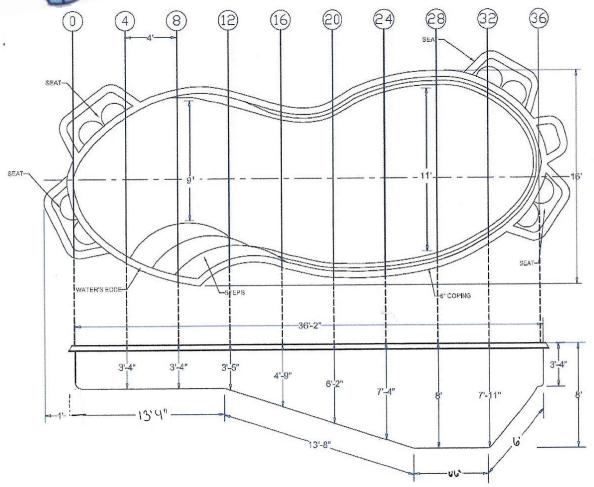
It is important to have your excavator call to review the Dig Diagram prior to excavation. All dimensions are Approximate. A 3" over dig must be added to the bottom for the stone, along with a 2' by 3' trench from the pool hole to the area of the equipment placement for plumbing and wiring.
