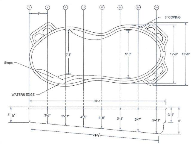
It is important to have your excavator call to review the Dig Diagram prior to excavation. All dimensions are Approximate. A 3" over dig must be added to the bottom for the stone, along with a 2' by 3' trench from the pool hole to the area of the equipment placement for plumbing and wiring.
