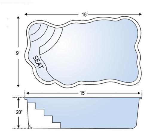
It is important to have your excavator call to review the Dig Diagram prior to excavation. All dimensions are approximate. A 3" over dig must be added to the bottom for stone, along with a 2' by 3' trench from the pool hole to the area of equipment placement for plumbing and wiring.
