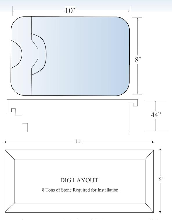
It is important to have your excavator call ahead and review the Dig Diagram prior to excavation. All dimensions are approximate. A 3" over dig must be added to the bottom for stone, along with a 2' by 3' trench from the bottom of the pool to the area of equipment placement for plumbing and wiring.
