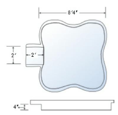
It is important to have your excavator call ahead and review the Dig Diagram prior to excavation. All dimensions are approximate. A 3" over dig must be added to the bottom for stone, along with a 2' by 3' trench from the bottom of the pool to the area of equipment placement for plumbing and wiring.
